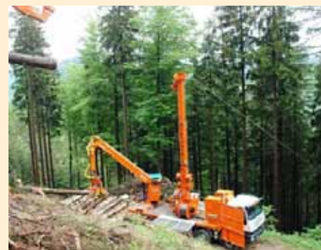
Application of the modern mobile cable crane on the forest harvesting
